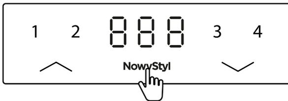
4. Measure the actual height, then use the “up” or “down” button to increase or decrease the number on the display until the actual height value is reached.
