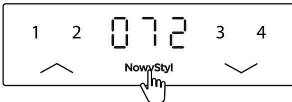
To exit the menu without making a selection, wait for about 10 seconds until the height value is shown on the display again.
