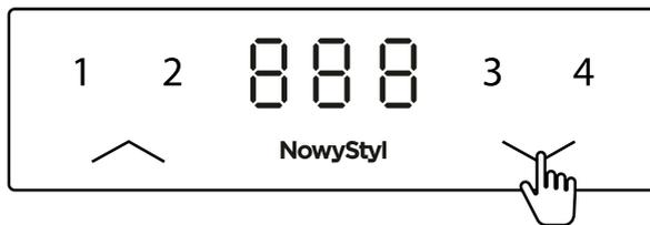
Press and hold the “**down**” button until the workstation reaches its lowest position, then release the button.
