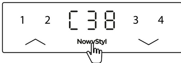
Default settings have been restored. The **C 38** symbol will be shown on the display. Finish by performing system Initialisation/First start-up (7.1).
