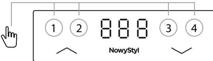
The height setting will be saved under the selected number, and a symbol will appear on the display, e.g. **P 1**. After approx. 2 seconds, the value of the saved height setting will appear on the display.
